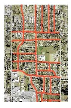
Decrease impermeable surfaces by narrowing roads, decreasing the number of driving lanes and re-paving with permeable material such as rubber popcorn or tile pavers. Trenches filled with mulch can absorb surface runoff and act as a base for street plantings. They can absorb 65-70% their volume in water
