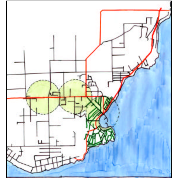
Arterials and street systems with 500m (5-minute walking distance) radius around major destinations.
